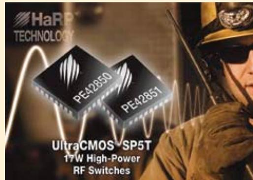
frequency range of 100 to 1000 MHz while the PE42850 extends the low end frequency to 30 MHz. Both Peregrine switches feature a low, mid-band insertion loss of 0.25 dB,
