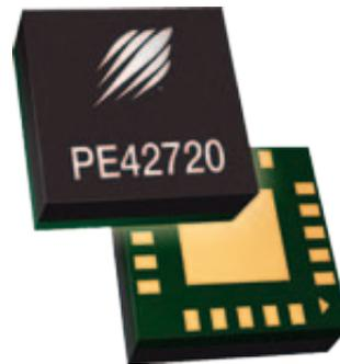
The PE42720 operates from 5 to 3000 MHz and is highly linear, delivering high isolation of 65 dB and low insertion loss of 0.7 dB at 1 GHz. It supports +1.8 V control logic and offers high ESD protection. Additionally, no blocking capacitors are required if DC voltage is not present on the RF ports. It is ideally-suited for supporting higher data rates in CATV applications, including CATV signal switching and distribution, cable modem headend, and DBS IF switching.
