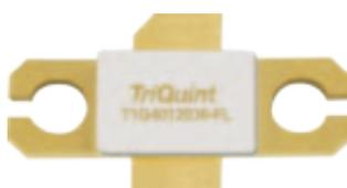
RFMW, Ltd. announced design and sales support for TriQuint Semiconductor wideband GaN on SiC transistors. The TriQuint T1G4012036-FL is a 120 W peak (24 W avg.) (P3dB) discrete transistor in a flange package while the TriQuint T1G4012036-FS provides an earless configuration. Both devices operate from DC to 3.5 GHz and offer > 50% drain efficiency from a 36V supply. Linear gain is as high as 15 dB. Both packages offer low thermal resistance and the
