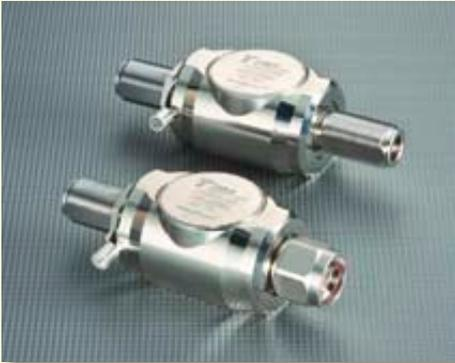
The Times-Protect LP-GPX-05-T high performance lightning protector is an exceptional DC pass design for protection of GPS receivers requiring up to 5Vdc power to be supplied on the center pin for L1, L2 and L3 bands. While the RF path is DC blocked, the biased DC voltage protection circuit uses state-of-the-art solid state protection technology to provide unsurpassed surge performance.
