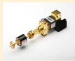
Spacek Labs model RE-15FISO is a full-band receiver which down-converts all of E-Band (60-90 GHz) to an IF of 2 to 32 GHz. The LO is derived from a mechanical tuned Gunn oscillator that provides 15 mW @ 58 GHz. **58**
