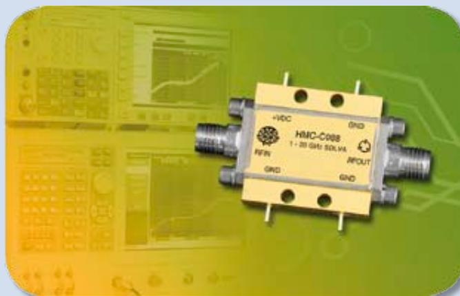
successive compression topology, which delivers a high logging range of 59 dB and allows for the processing of high level signals up to  $+5$  dBm. During typical operation, the HMC-C088 provides a nominal slope of 14 mV/dB and a typical intercept of  $-119$  dBm at 10 GHz.
