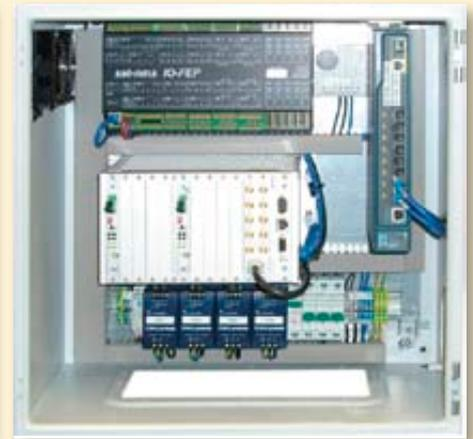
SatService GmbH developed a new member of its successful fibre optical transmission systems. The presented Optical Link Outdoor Cabinet will provide the safe environmental home for Qty 10 or 20 of the proven sat-nms LFTX and LFRX modules. The same modules can be used in this outdoor application and also in the existing indoor 19" rack mount chassis. The cabinet can be equipped with optical converters only or is can include also other satellite ground sta-
