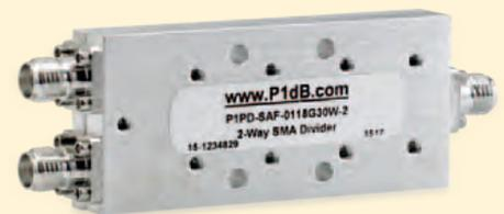
P1dB, an RF and Microwave component supplier, released a new ultra-broadband 2-way SMA power divider operating from 1 to 18 GHz. The P1PD-SAF-0118G30W-2 SMA power divider is a Wilkinson RF splitter that is capable of handling 30 watts of RF power. The RF power divider is in stock and is available at P1dB.
