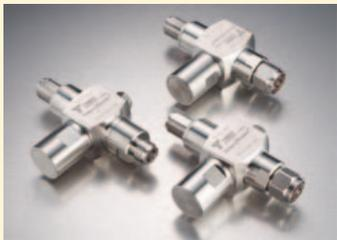
The new LP-STRH series is part of the Times-Protect line of innovative RF lightning and surge protection products. The LP-STRH series is an exceptional DC blocked design with outstanding surge performance designed for the new LTE (Long Term Evolution) and Public Safety requirements in the 700 to 2700 MHz range.
