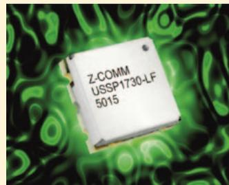
Z-Communications Inc. announced a new RoHS compliant VCO (Voltage Controlled Oscillator) model USSP1730-LF in the L-band. The USSP1730-LF operates from 1715 to 1745 MHz within a tuning voltage range of 1 to 4 V<sub>DC</sub>. This remarkable VCO features phase noise of -94 dBc/Hz @ 10 kHz offset while operating off a 5 V supply and typically drawing only 19 mA of current.
