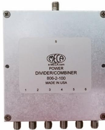
Meca Electronics announced non-binary 3 & 6-way broadband power dividers optimized to cover 1.5 to 2.7 GHz (803-2-2.100 & 806-2-2.100) encompassing various aeronautical, satellite and mobile bands. With typical performance of SWR of 1.2, isolation 27 dB, insertion loss 0.6 dB and exceptional amplitude & phase balance of 0.3 dB & 6 degrees max. This is in addition to the family of 2, 3, 4, 8, 9, 12 & 16 way splitters. Made in the USA and 36 month warranty.
