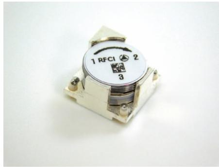
ture range. Ideally suited for high-volume manufacturing, these circulators are available on tape and reel and may be ordered in clockwise or counter-clockwise rotation.
