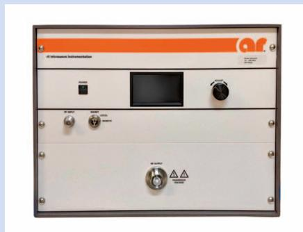
failure. The Model 600A400 is equipped with a Digital Control Panel (DCP) which provides both local and remote control of the amplifier. The DCP uses a color LCD touch screen display to indicate the operate status and fault conditions if an overtemperature or power supply fault has occurred. The unit can be returned to operate when the condition has been cleared.
