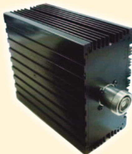
features low PIM performance of <math><163\text{ dBc}</math> @ +43 dBm/ tone. VSWR performance is 1.09:1 from a 7/16 female connector. The P1LP-Term-716J100W from P1dB continues the expansion of P1dB's family of Low PIM offerings, including cable assemblies, adapters, attenuators, and now terminations. The P1LP-Term-716J100W is well suited for a variety of base station
