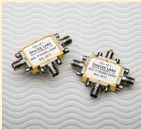
Space Labs Model P1M29B3-2208F is a compact (1.0" x 1.6" x 0.3"), economical and high-performance K-band mixer in the PM Series. With a high IF bandwidth of up to 13 GHz, the full RF/LO range is available in a single unit. This double balanced mixer design performs with a flat-response con-
