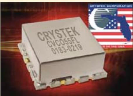
Crystek's CVCO55FL-0183-0219 VCO operates from 183 MHz to 219 MHz with a control voltage range of 0.5 V ~ 4.5 V. This VCO features a typical phase noise of -123 dBc/Hz@10 kHz offset and has excellent linearity. Output power is typically +8.5 dBm.
