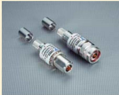
Times Microwave Systems introduces the new Times-Protect LP-18-400-N series of DC pass RF lightning and surge protection products with a frequency operating band from DC to 6000 MHz. This new bidirectional design with either a type N male or type N female connector on one end can be directly attached to LMR-400 cable via the same standard EZ non-solder interface
