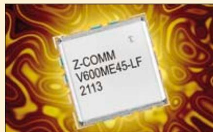
Z-Communications, Inc. announced a new RoHS compliant VCO model V600ME45-LF ideal for satellite communication applications. The V600ME45-LF operates from 3000 to 6000 MHz with a tuning voltage range of 0-24 Vdc. This octave tuning VCO features a typical phase noise of -103 dBc/Hz @ 100 kHz offset and an average tuning sensitivity of 147 MHz/V.
