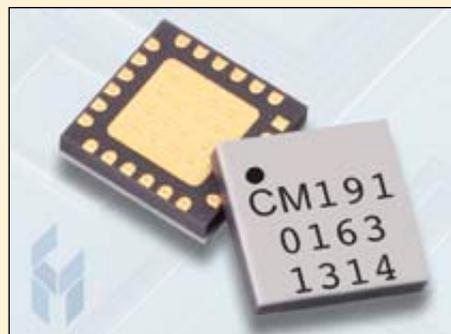
eliminates the need for external DC blocks and RF port matching. The CMD191C4 is biased with a single 5.0 V positive drain supply. RF power can be applied at any time. Suitable applications include WLAN, C and X Band communications systems and military end-use.
