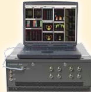
Agilent introduced industry-leading enhancements to its N7109A multi-channel signal analyzer for emerging multichannel LTE, LTE-Advanced and MIMO RF measurement requirements, including LTE antenna beamforming and LTE-Advanced carrier aggregation. **56**
