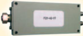
RLC Electronics' manually adjustable delay line (phase shifter) offers continuous adjustment of electrical delay over the frequency range of DC - 40 GHz. Adjustment is through a multi-turn, locking shaft. Low insertion loss and VSWR are maintained throughout the adjustment range. The unit comes with a choice of male or female 2.92 mm connectors.
