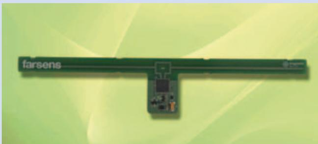
The Magneto from Farsens S.L., San Sebastián, Spain, is a battery free RFID sensor tag capable of transmitting a unique identifier and the associated magnetic field measurement data to a commercial EPC C1G2 reader without the need of a battery on the sensor tag.
