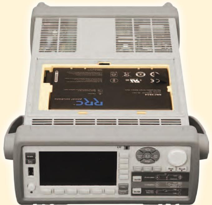
The B2980A Series battery operation model (B2983A/B2987A)
