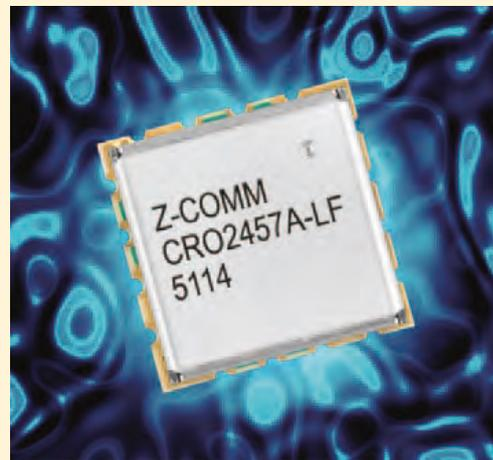
Z-Communications, Inc. announces a new RoHS compliant VCO (Voltage Controlled Oscillator) model CRO2457A-LF. The CRO2457A-LF operates at 2457 to 2458 MHz with a tuning voltage range of 0.5 to 4.5 VDC. This high performance VCO features a spectrally clean signal of -115 dBc/Hz @ 10 kHz offset and a typical tuning sensitivity of 8 MHz/V. The CRO2457A-LF is designed to deliver +6 dBm of output power into a 50 ohms load while operating off a 5 VDC sup-
