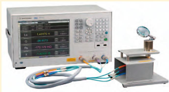
Keysight Technologies, Inc. today introduced three low-frequency options for its E4982A LCR meter. With these new options, the E4982A is well suited for RF inductor, coil and EMI filter manufacturers that are required to perform impedance testing at various frequencies.
