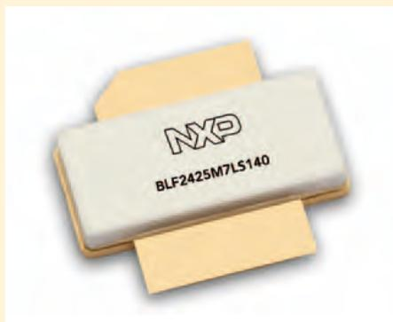
RFMW, Ltd. announced design and sales support for an LDMOS power transistor internally matched for broadband operation from 2.4 to 2.5 GHz. NXP's BLF-2425M7LS140 provides 140 W average CW power with 18.5 dB of gain. The BLF-2425M7LS140 draws 1.3 A from a 28 V supply with efficiencies up to 52%. Housed in a ceramic package with solder ears, the
