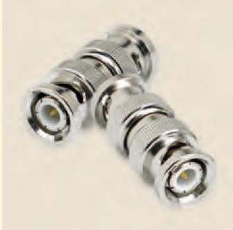
RFMW Ltd. announced design and sales support for model P1AD-BNMM from P1dB. The P1AD-BNMM is a BNC male to BNC male adapter offering a miniature, quick connect/disconnect for commercial RF applications. Operating up to 3 GHz in a 50 ohm environment, the adapter's body is nickel plated zinc while the center contacts are gold plated brass. The P1AD-
