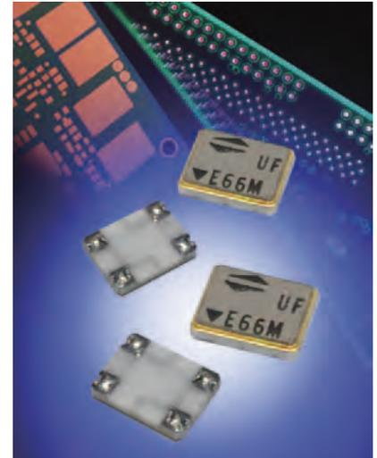
Euroquartz has launched a new range of low-power ultra-miniature quartz crystal oscillators from Statek designed for use in a wide range of applications. Hermetically sealed in a high reliability 4-pad ceramic surface mount housing, the new oscillator offers fast start-up of 1 ms typical, tight calibration tolerance of  $\pm 25$  ppm and high shock resistance of 10,000 g typical.
