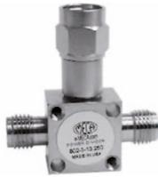
band Resistive Power Splitters covering DC-18 GHz (802-3-9.000) and DC-26.5 GHz (802-3-13.250) encompassing VHS thru X & Ku bands. With typical performance of: SWR 1.3, Insertion Loss 1.5 dB and exceptional Amplitude & Phase Balance of 1 dB & 4 degrees max. Made in the USA, 36 month warranty.
