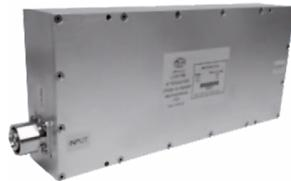
MECA offers Broad Band Low PIM Attenuators 50 watt models with a Typical PIM spec of -161 dBc. Featuring 4.1/9.5, 7/16, N and 4.3/10.0 DIN interfaces with custom in-between styles also available upon request. Covering 600 MHz through 4 GHz. While handling full rated power to 85 °C with no derating. Made in USA and 36-month warranty.
