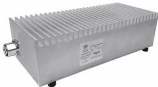
MECA offers Broad Band Low PIM Attenuators 100 watt models with a typical PIM spec of -161 dBc. Featuring 4.1/9.5, 7/16, N and 4.3/10.0 DIN interfaces with custom in-between styles also available upon request. Covering 600 MHz through 4 GHz. While handling full rated power to 85 °C with no derating. Made in USA and 36-month warranty.
