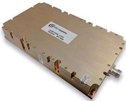
comm. Model number SSPA 0.2-2.5-200 operates from 200 to 2500 MHz and delivers a typical, saturated output power of 200 W. Designed and tested to withstand MIL-STD-810 high shock and vibration requirements, small signal gain is ~60 dB and operating voltage is 50 V DC. The SSPA 0.2-2.5-200 is offered in a modular housing that is approximately 5" (width) by 9" (long) by 1.5" (height). The RF input connector is SMA female and the RF output connector is Type N female.
