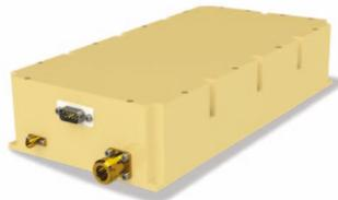
Typical small signal gain is 53...55 dB. Operating from a 28 V supply, this amplifier includes an external DC blanking command that enables and disables the module in less than 10  $\mu$ s. Offered in a modular housing that is approximately 5" (width) by 9" (long) by 2" (height).
