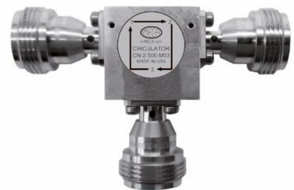
Meca Electronics' latest product offering: compact circulators covering 2.1...2.7 GHz N & SMA interfaces encompassing PCS & DCS bands. Typical specs: SWR of 1.2, isolation 23 dB and insertion loss 0.3 dB in
