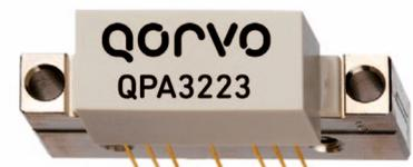
RFMW, Ltd. announced design and sales support for a low current hybrid amplifier. Qorvo's CATV power doubler model QPA3223 reduces system DC current requirements as it draws only 410 mA from a 24 V supply. However, performance remains high due to the combination of GaAs pHEMT and GaN pHEMT die providing 21 dB minimum gain from 45 to 1003 MHz (23 dB typical @ 1003 MHz). Return loss is >17 dB for
