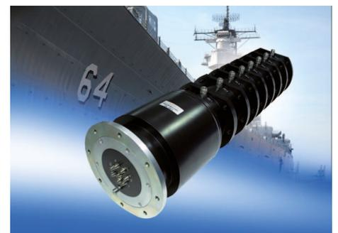
Link Microtek has designed and produced a complex 700 mm long 8-channel coaxial rotating joint for use in an L-band shipborne long-range radar system. Enabling microwave signals to be fed to and from the radar antenna, the rotating joint features six PSR (primary surveillance radar) channels, each with a frequency range around 1400 MHz, and two SSR (secondary surveillance radar) channels covering frequencies between
