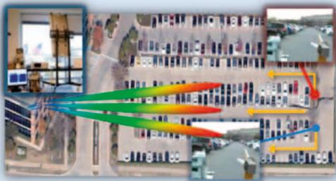
**Figure 4: Samsung FD-MIMO 3D beamforming prototyping system implemented with four NI USRP RIO software receivers**
