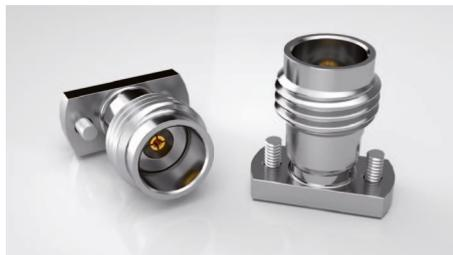
Samtec announced the release of their new 2.4 mm Compression Mount Connector designed to perform to 50 GHz. Primarily for use in the highspeed digital test market this connector is designed for stripline applications. The connector is vertically mounted to the PCB and attached in place by two 0-80 UNF screws eliminating the need for soldering to the test points. Microstrip design in development.
