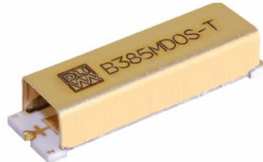
pass band. Measuring 6.985 x 2.032 mm, this surface mount filter offers 2.5 dB typical insertion loss with 40 dB out-of-band rejection. Catalog devices come complete with integrated shielding and the surface mount versions are designed for use on most RF PWB materials.
