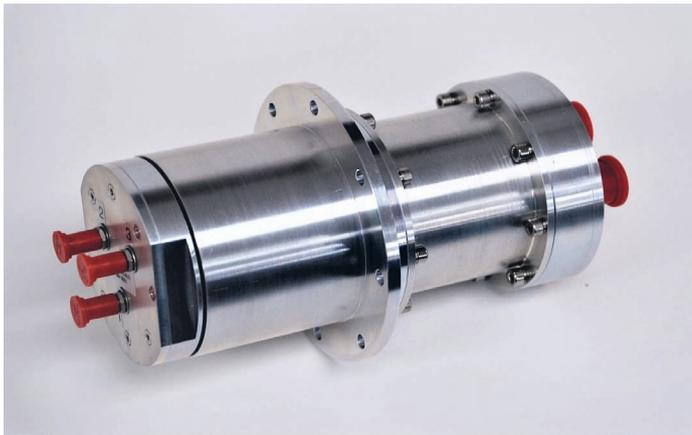
The latest addition to Link Microtek's extensive range of microwave rotary joints is a device featuring three X-band channels, one of which is used for transmit and the others for receive signals in radar systems for coastal/border surveillance or critical infrastructure protection. Designed and manufactured at Link Microtek's facility in Basingstoke, UK, the
