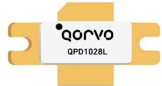
RFMW announced design and sales support for a high power GaN transistor from Qorvo. The QPD1028L delivers >750 W of saturated power from 1.2 to 1.4 GHz for military and civilian L-Band radar systems. Efficiency at Psat is 67 to 70% with 17 to 18 dB of gain. The QPD1028L is capable of CW or pulsed operation with 65 volt bias. This input-pre-matched device is housed in an industry standard air cavity package.
