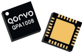
RFMW announced design and sales support for a variable gain amplifier (VGA) from Qorvo. The QPA1008 is a two-stage variable gain amplifier for S-band applications from 2.7 to 3.8 GHz. It includes a 30 dB analog attenuator and resistively coupled power detector at the output for circuits requiring power monitoring. <20 ns bias switching for quick turn-on/turn-off operation improves system sensitivity in commercial and military radar, communications systems and test & measurement applications.
