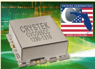
Crystek's VCO (Voltage Controlled Oscillator) CVCO55CC-1290-1310 operates from 1290 to 1310 MHz with a control voltage range of 0.5 to 4.5 V. This VCO features a typical phase noise of -117 dBc/Hz @ 10 kHz offset and has excellent linearity. Output power is typically 1 dBm.
