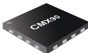
RFMW announced design and sales support for two MMIC power amplifiers from CML Microcircuits. The CMX90A003 and CMX90A004 are two-stage, fully matched MMIC power amplifiers for use in 860 to 960 MHz, license-free bands. Advanced GaAs HBT techno-
